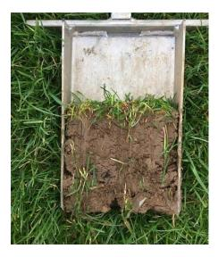
The soil results analysed showed less than 20% beneficial drainage sands in them (coarse and medium sand content). The high levels of the finest particles (clay and silt) amounting to 49% of the sample. The rest of each sample was made up of fine and very fine sands which are classified by sieve size and will compound drainage issues and compaction further.
